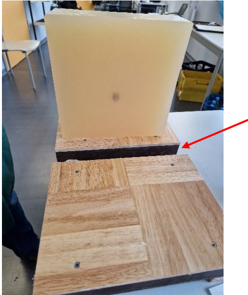
Figure 6: Laboratory table with cutting support and an already cut soap block. The support surface is open in the middle (see arrow) to allow complete cutting. The picture further shows that the block was cut just behind the stuck bullet.
