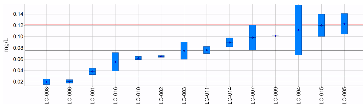
Figure 10: Measurement result range reported by the participants for the third release test of Co into 3 % acetic acid (2h at 70°C). Red lines demonstrate z score = 2 ( x_{pt} \pm 2 \sigma_{pt} ), black line is x_{pt} , points and bars show x_i and U_i
