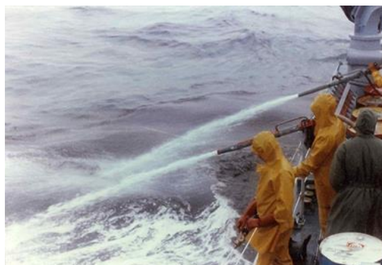
Figure 4.7: Use of fire hoses for dispersant spraying in the Amoco Cadiz casualty. In retrospect, the lack of efficient flow control did not enable application according to the use recommendations. (source: Cedre).
