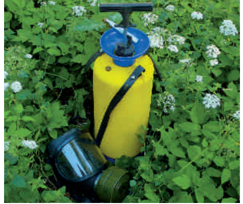
Fig. 24: Knapsack sprayer with protective mask for the application of pesticides
